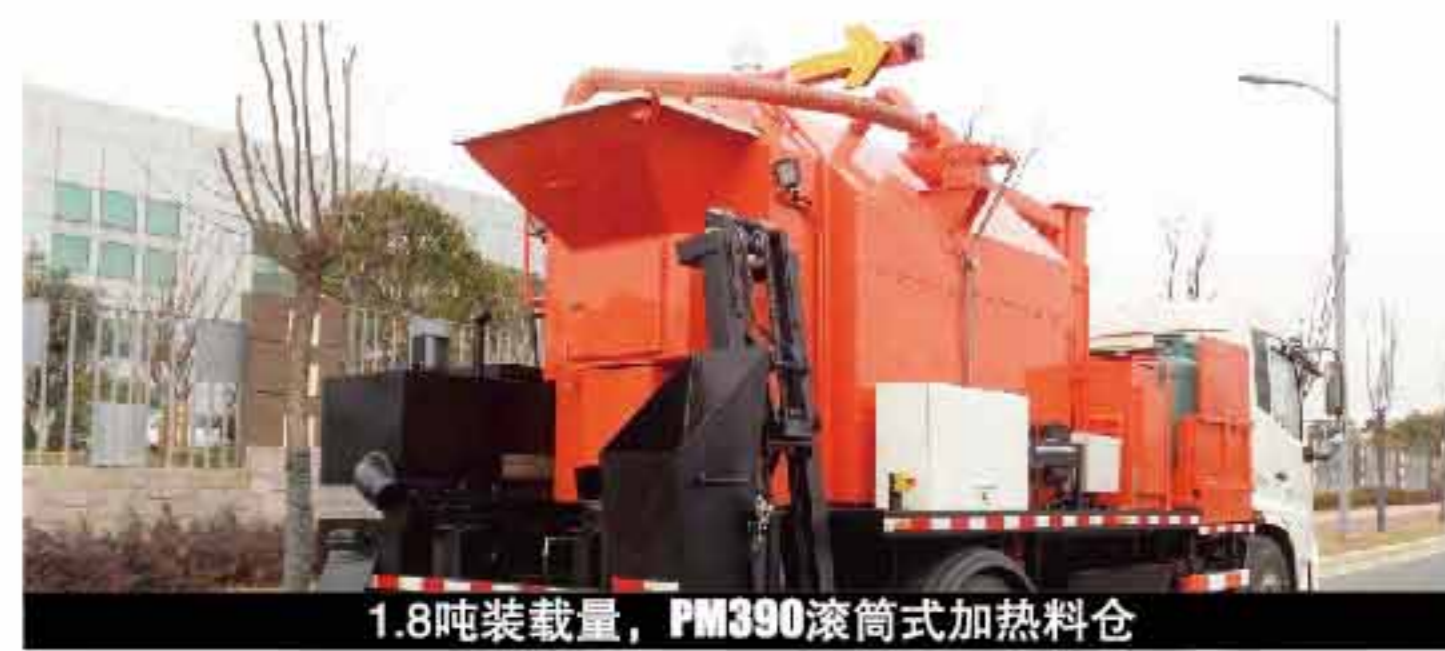
1.8吨装载量, PM390滚筒式加热料仓
